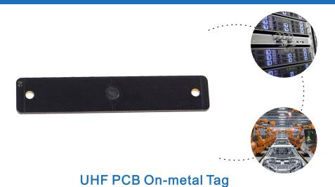
The tag is based on FR-4 materials with IP68 rated, it has super reliability and durability, high temperature resistant, suitable for different harsh environments. It could be installed via screw, rivet, adhesive, etc and it is compitable with the protocol ISO18000-6C (EPC C1G2) with unique global ID, suitable differet assets tracking
