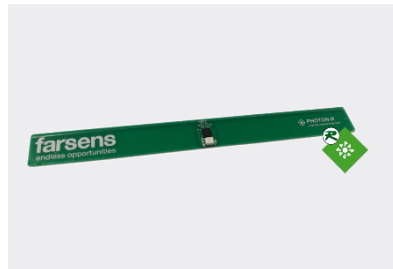
RF Field Monitoring Sensor Tag
