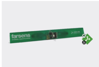
Three-axis Acceleration Sensor Tag
