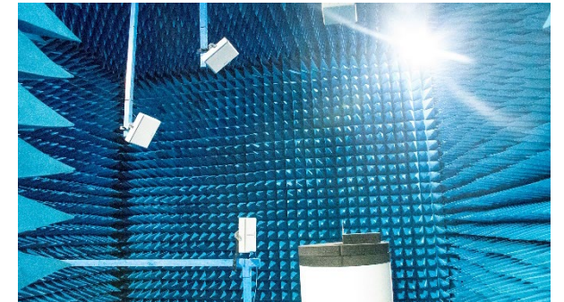
RFID Anechoic room
